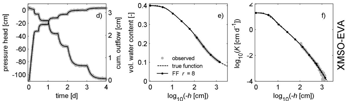
**Fig. 6:** As Fig. 5, but using a free-form model of hydraulic properties in the parameter identification.
