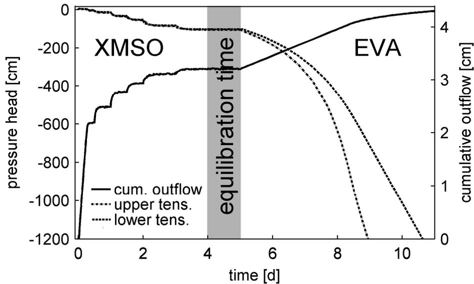
Fig. 3: Cumulative outflow (from lower left to upper right) and pressure heads at 1.8 and 5.4 cm height levels (from upper left to lower right) inside a 7.2 cm high soil column during the consecutive extended multistep-outflow (XMSO) and evaporation (EVA) experiments for a loam soil (synthetic data).
