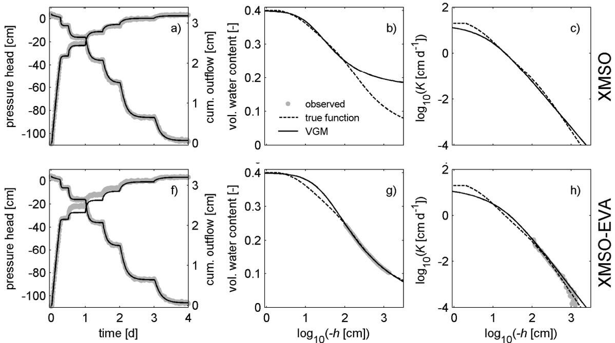
**Fig. 5:** Results from the individual extended multistep-outflow (XMSO, top) and from the combined (XMSO-EVA) experiment (bottom) for a loamy soil and the van Genuchten-Mualem (VGM) parameterization. Left: measured and fitted values for cumulative outflow and pressure head at 1.8 cm below the top (XMSO). Middle and right: true and estimated  $\theta(h)$  and  $K(h)$  functions and data points from the simplified EVA method.
