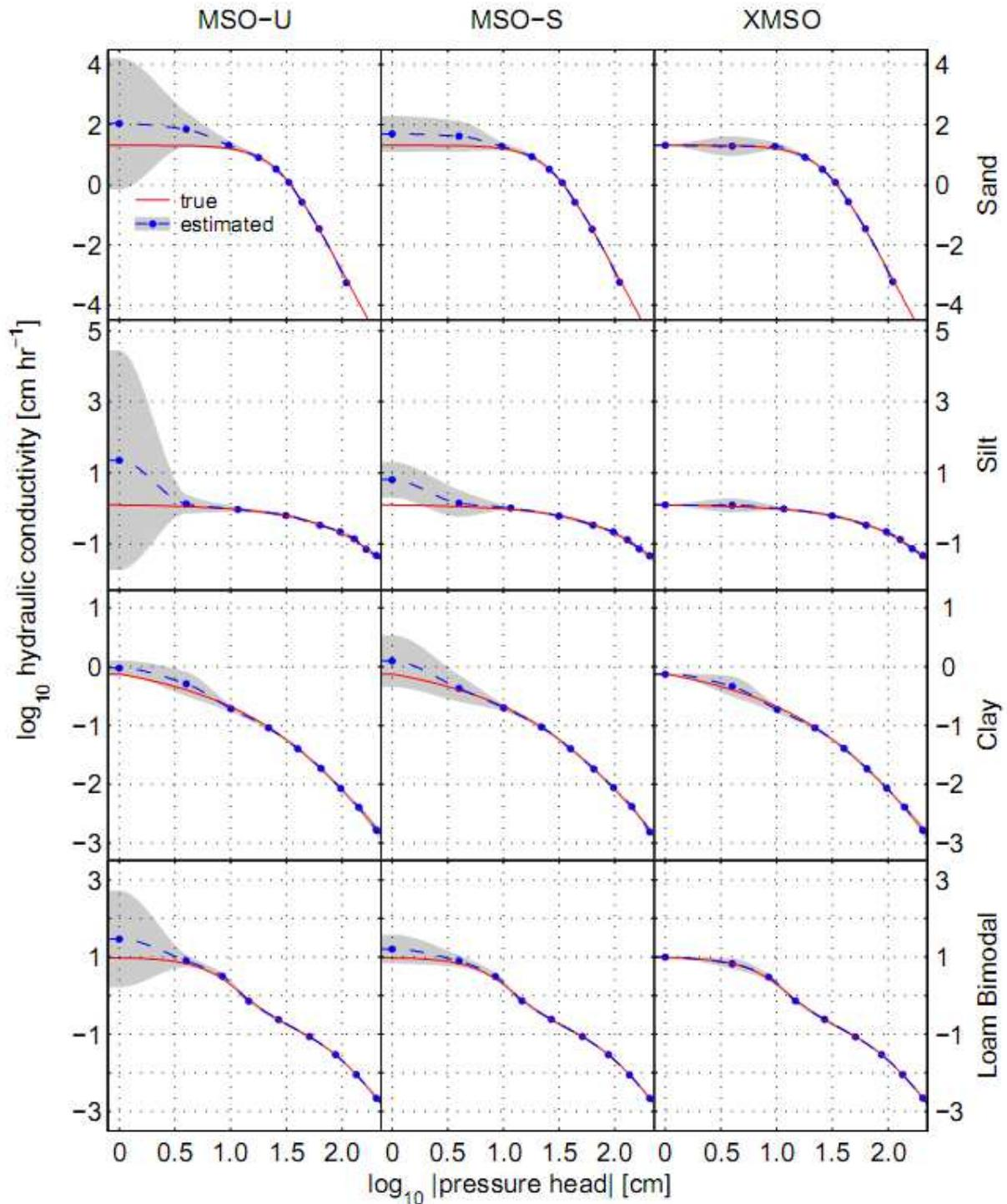
**Fig. 4:** Unsaturated hydraulic conductivity functions estimated using the free-form parameterization for the synthetic data sets and the known true functions. The grey-shaded areas visualize the 95%-confidence band of the estimated functions. Points used for cubic Hermite interpolation are denoted as blue dots.
