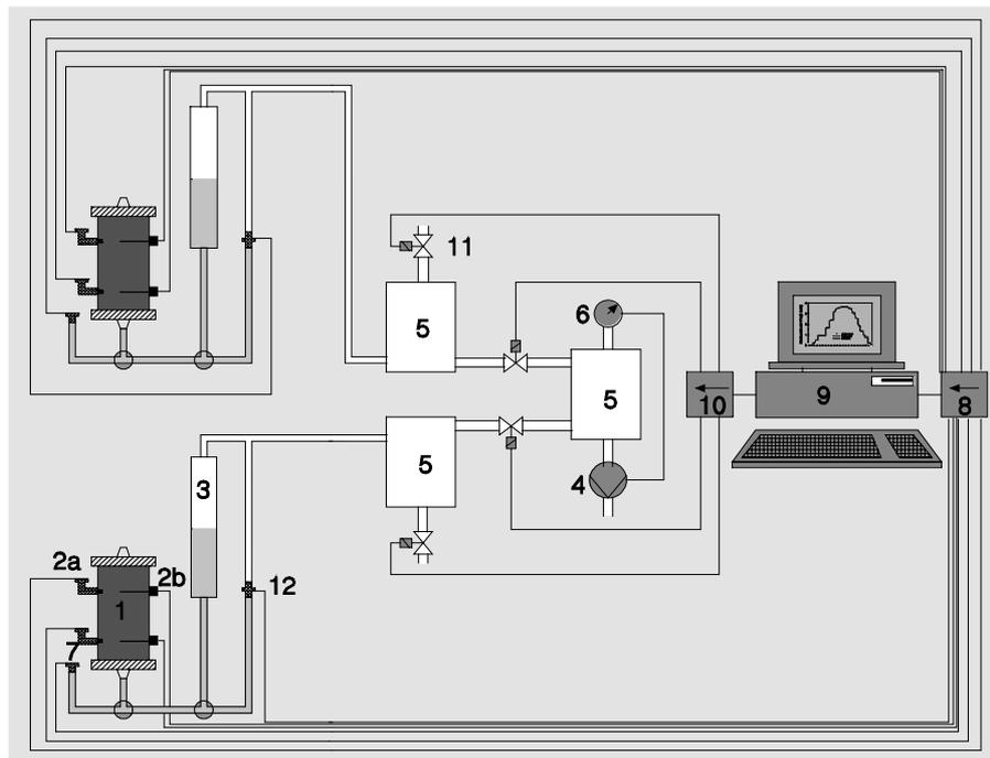
Fig. 3. Schematic of the experimental device: (1) soil core, (2a) microtensiometer with pressure transducer, (2b) TDR, (3) burette, (4) vacuum pump, (5) storage bin, (6) manometer, (7) pressure transducer, (8) multiplexer and analog/digital converter, (9) computer, (10) digital/analog converter, (11) magnetic valve, and (12) difference pressure transducer.
