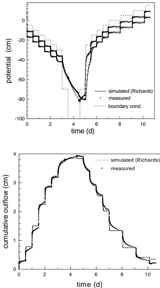
Fig. 1. Measured and simulated outflow and backflow during a multistep experiment on undisturbed Forchheim sand. Left: Tensiometric potential (measured), matric potential (simulated) and pressure at the lower boundary. Right: Cumulative water flow.
