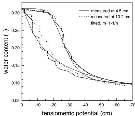
Fig. 2. In-situ measured retention curves of a sample of Forchheim sand during a multistep drainage and imbibition experiment.
