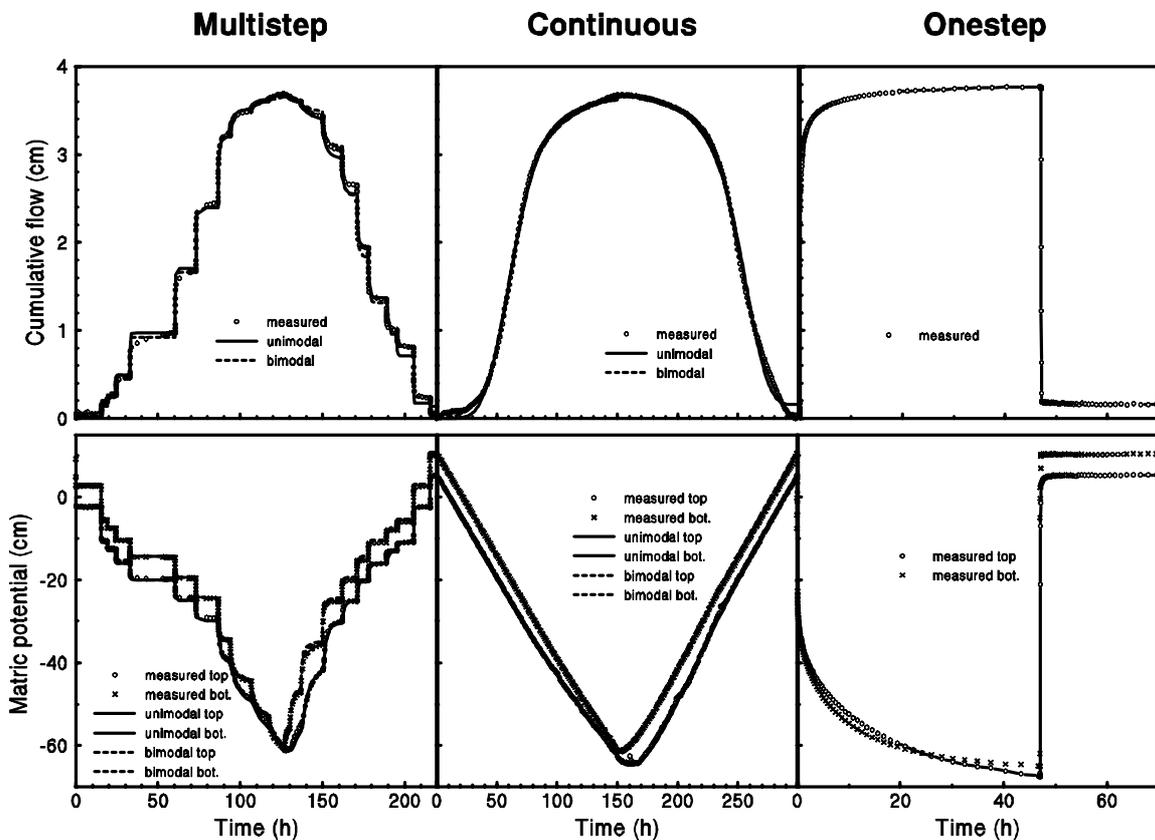
Fig. 1: Simulated and measured outflow and inflow curves and tensions for the experiment.
